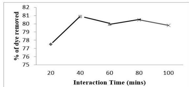
Fig. 2. Impact of Interaction Time on the adsorption of the dye by avocado pear seed adsorbent
