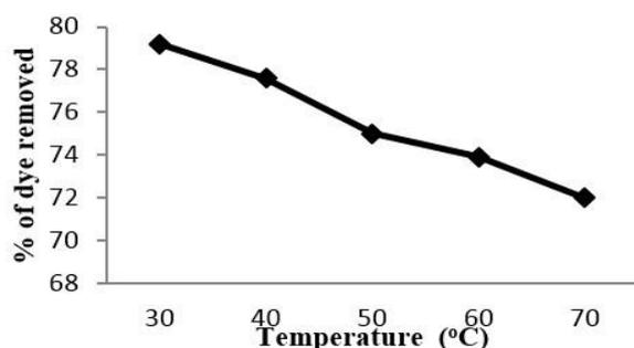
Fig 5. Impact of temperature on the adsorption of the dye by avocado pear seed
