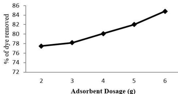
Fig 3. Impacts of adsorbent dosage on the adsorption of the dye by avocado pear seed
