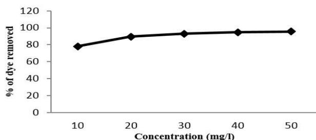
Fig. 4. Impact of concentration on the adsorption of the dye by avocado pear seed
