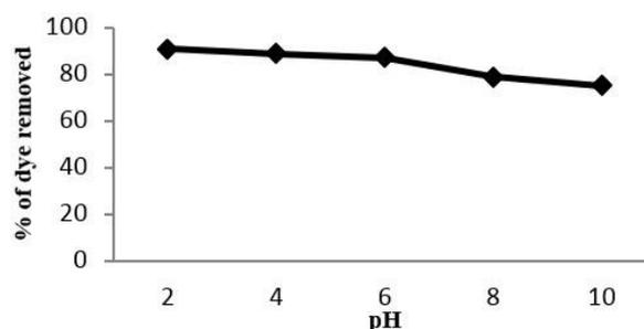
Fig. 6. Impact of pH on the adsorption of the dye by avocado pear seed
