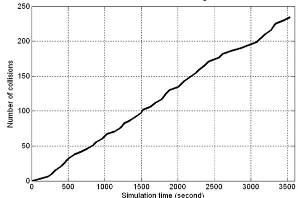
Fig. 7. The average of collision status of slotted Aloha protocol in UAN
