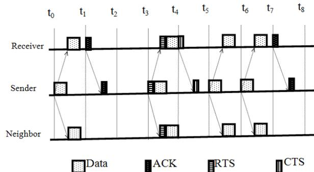
Fig. 3. A successful transmission of a single data packet and data packets train of slotted Aloha-FAMA
