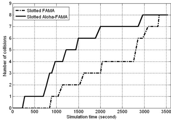
Fig. 8. The average of collision status of slotted FAMA and slotted Aloha-FAMA protocols in UAN
