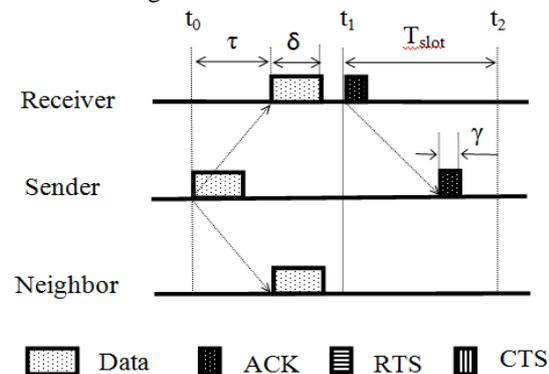
Fig. 1. A successful single data packet transmission of slotted Aloha protocol
