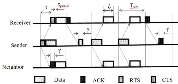
Fig. 2. A successful handshake of slotted FAMA protocol
