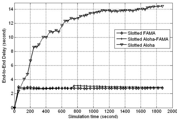
Fig. 9. The average of End-to-End delay of slotted Aloha, slotted FAMA, slotted Aloha-FAMA protocols in UAN
