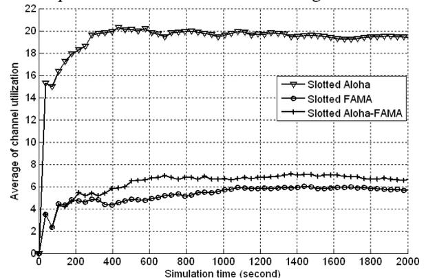
Fig. 6. The average of channel utilization of slotted Aloha, slotted FAMA, slotted Aloha-FAMA protocols in UAN
