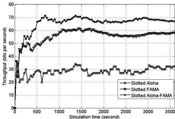
Fig. 10. Throughput of slotted Aloha, slotted FAMA and slotted Aloha-FAMA protocols in UAN
