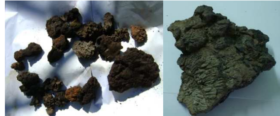
Fig. 1. Samples of iron slag from various portions of the smelting site at Tumbu Ching, Manipur (left). A large molten matrix of one such sample (right)
