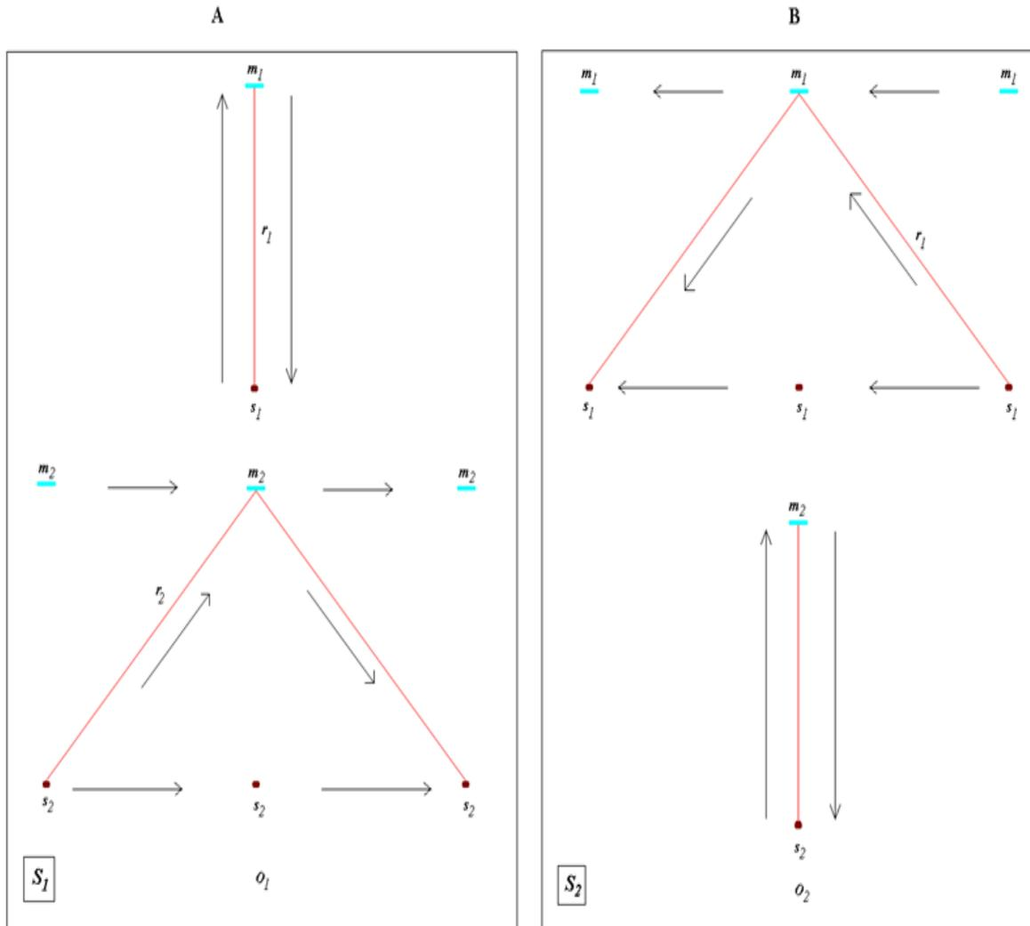
Fig. 1. In A the observer  $O_1$ , the light source  $s_1$  and the mirror  $m_1$  are at rest in  $S_1$ . A light pulse  $r_1$  goes from  $s_1$  to  $m_1$  and then from  $m_1$  to  $s_1$ . Another light pulse goes from the light source  $s_2$  to the mirror  $m_2$  and then from  $m_2$  to  $s_2$ ;  $s_2$  and  $m_2$  are moving to right with respect to  $O_1$ .
