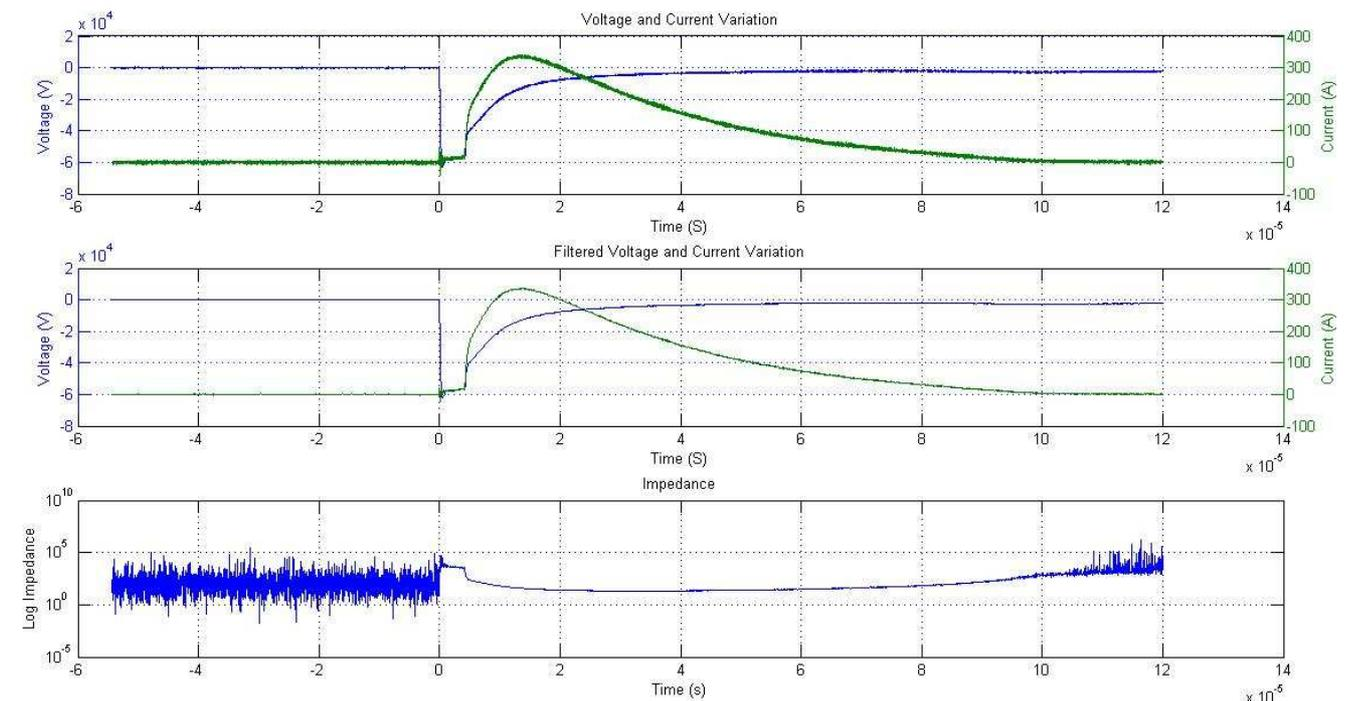
Fig. 6. Impedance characteristics of Soil Negative voltage impulse
