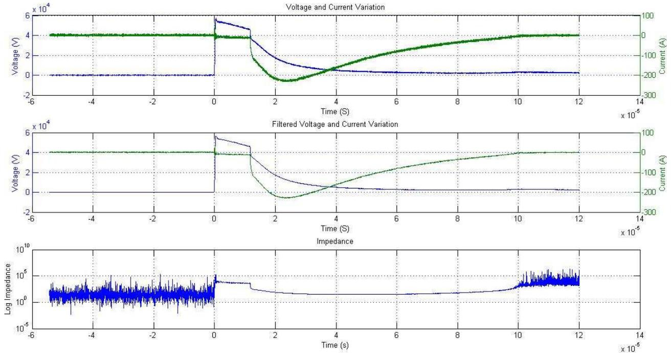
Fig. 5. Impedance characteristics of Soil Positive voltage impulse
