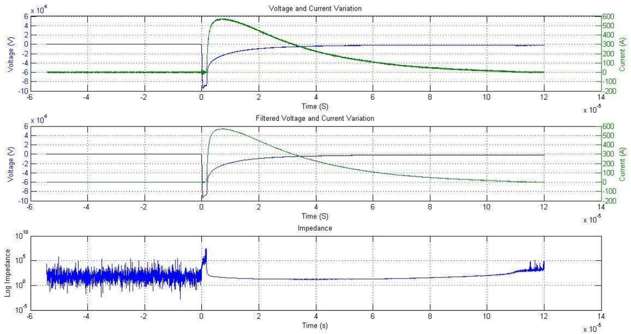
Fig. 4. Impedance characteristics of Sand Negative voltage impulse
